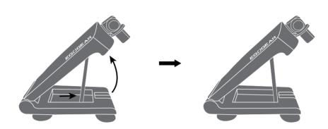
2 Push the wheel connector upward until the fixation button pops back into position.
