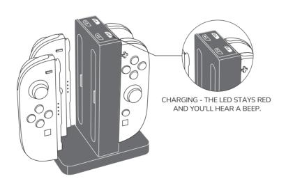
\* The product features a built-in magnetic function that automatically secures the handles when inserted into the charging slots.
