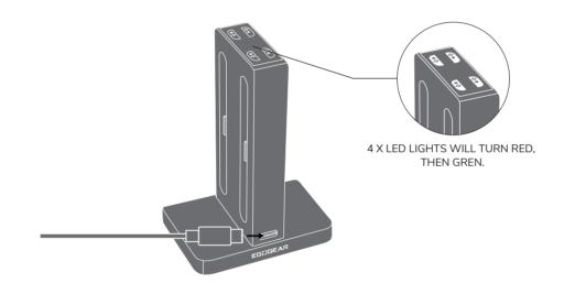
Insert your Joy-Con™ 2 controllers into the 4 charging slots. Make sure each one is properly connected.
